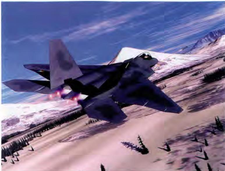
Stealth makes an object become very difficult to detect by sensors such as radar, heat seekers (infrared), sound detectors, and even the human eye. While not invisible, the F-22's radar cross section is significantly smaller when compared to other current fighters making it difficult for enemy radars to detect.
